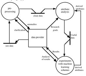
Figure 1: Process model for a machine learning application
