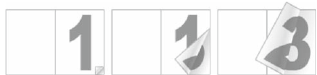
Fig. 2 Page turning using a two-dimensional geometric model
